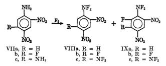
Fluorination of the *ortho* positions can occur through the reaction of intermediate stabilizing radicals such as X or XI shown below with fluorine followed by abstractions of the *ortho* hydrogen and continued fluorina-
